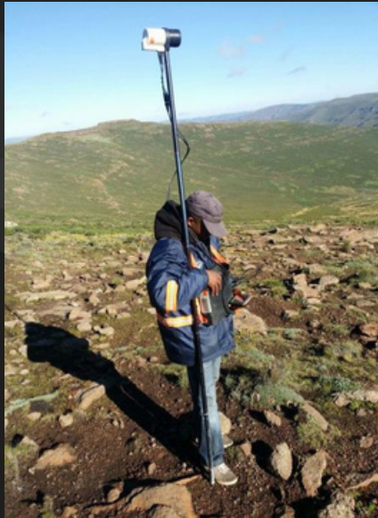
Fig 5: Magnetic data acquisition using the GSM-19 magnetometer (left) and fine-grained kimberlite with phlogopite flakes (Sources: MSA & MAMINO)
