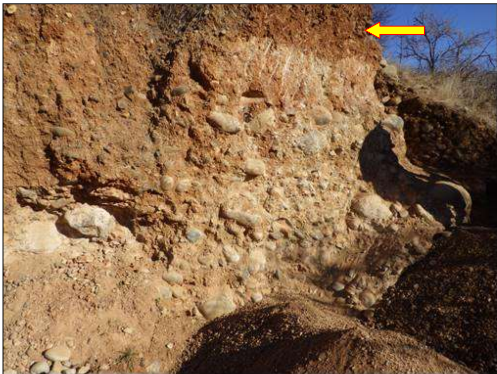
Photo 12. Artisanal digging upstream from confluence of the two Harts rivers (Near sampling point BB/07 - Figure 7). Overburden ~ 1 m; gravel > 2m. Note ~ 0.5 m layer of Rooikoppie gravel (arrow).
