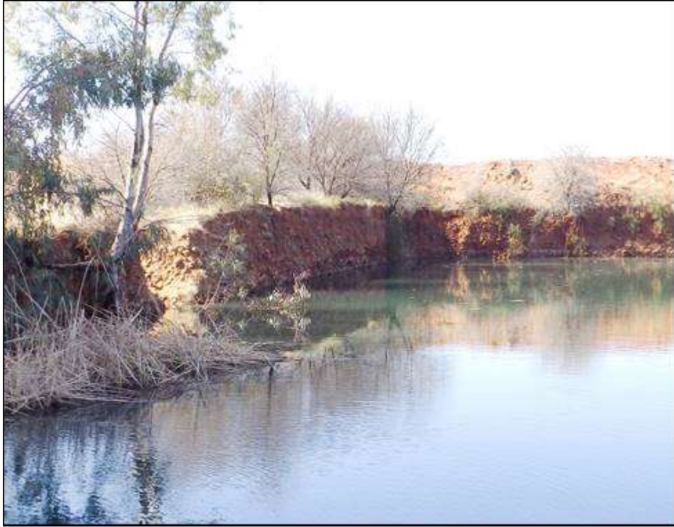
Photo 9. Flooded pit used as water source for BB3 operation. Overburden ~ 0.5 m, gravels ~ 3.5 m.
