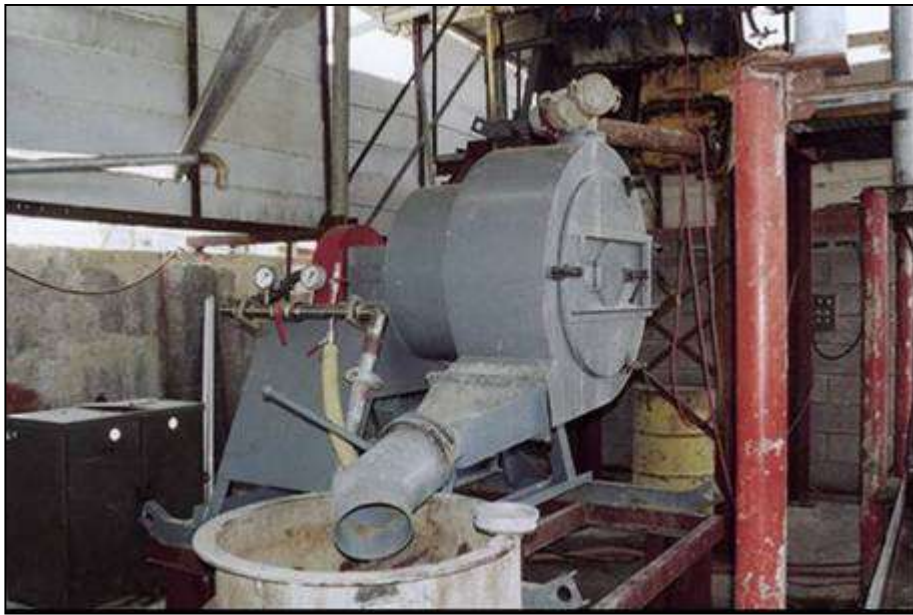
Photo 18. ITOMAK-KGM2-20,0 Centrifugal concentrator (20 ton/hour).
