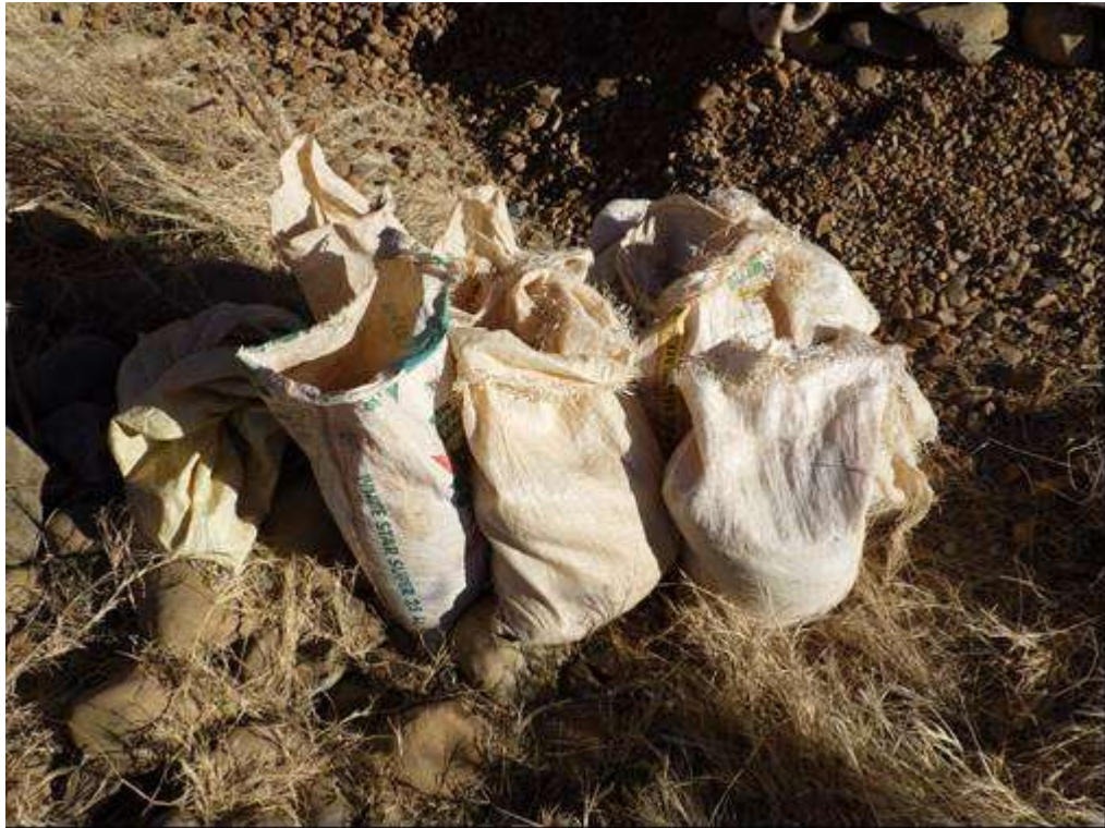
Photo 13. Bags filled with sieved gravel to be transported to the river for washing.
